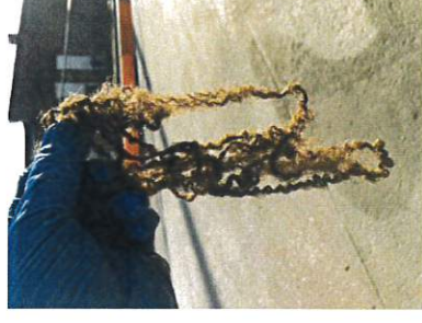
Tank bottom debris removed during fuel restoration project
